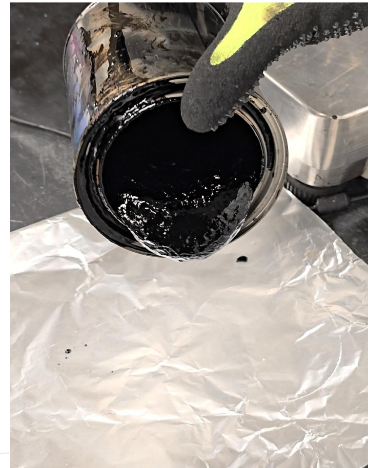
Poor workability with phase separated plastic modified asphalt binder
