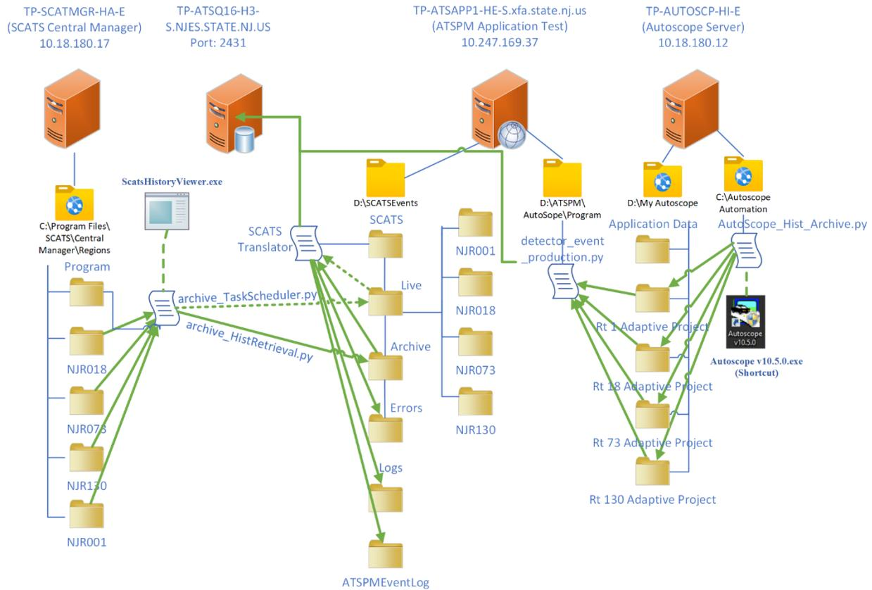
Figure 39. SCATS, Autoscope, and ATSPM Deployment Diagram
