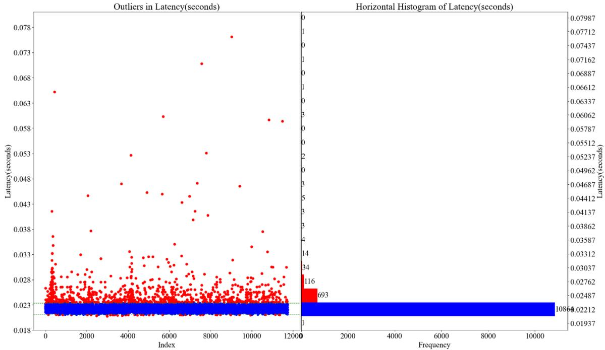
Figure 20. PSM Message Latency Analysis Results for 60 Minutes
