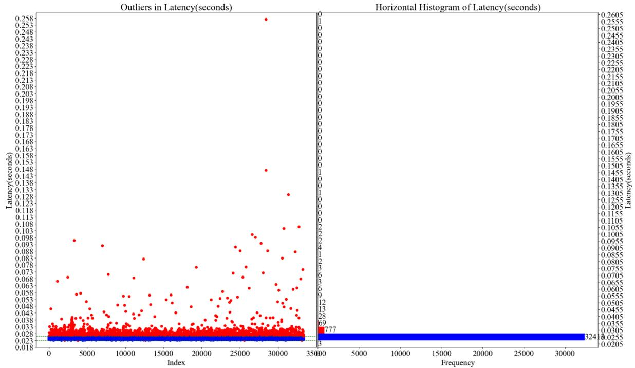
Figure 19. SPaT Message Latency Analysis Results for 60 Minutes
