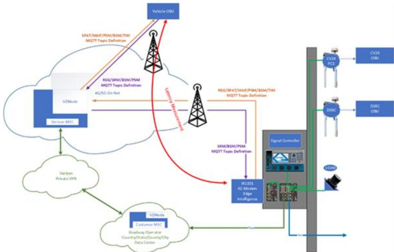
Figure 46. Illustration of Virtual RSU (vRSU) Deployment at NJDOT Test Site in Bordentown, NJ
