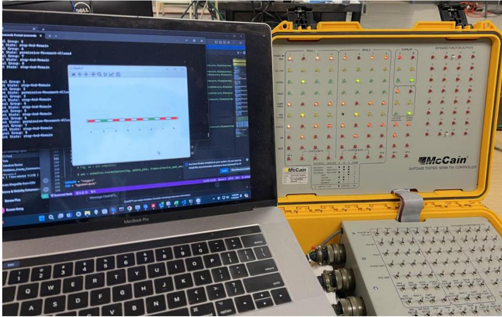
Figure 63. SPaT Message Visualization (Left: Received Message, Right: controller)
