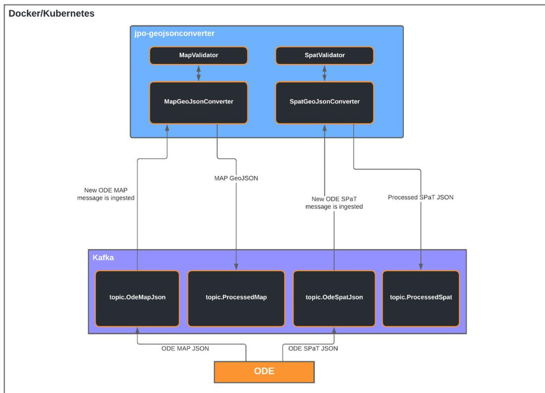
Figure 26. GeoJson Converter Architecture
