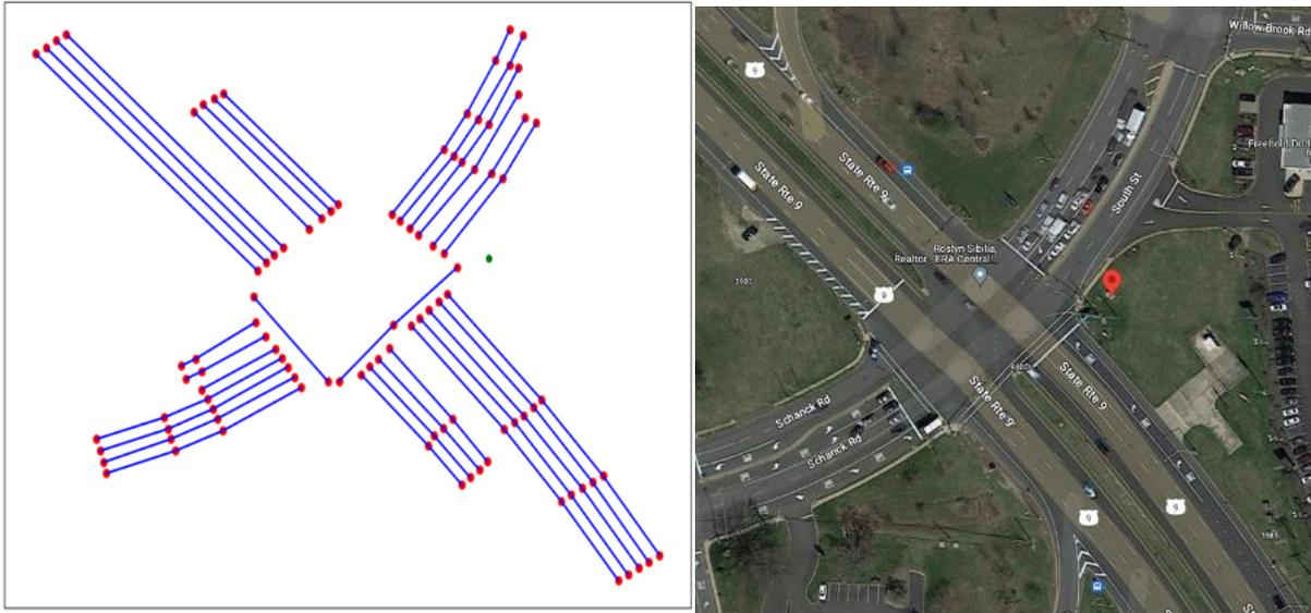
Figure 32. MAP message Visualization on Tested Intersection
