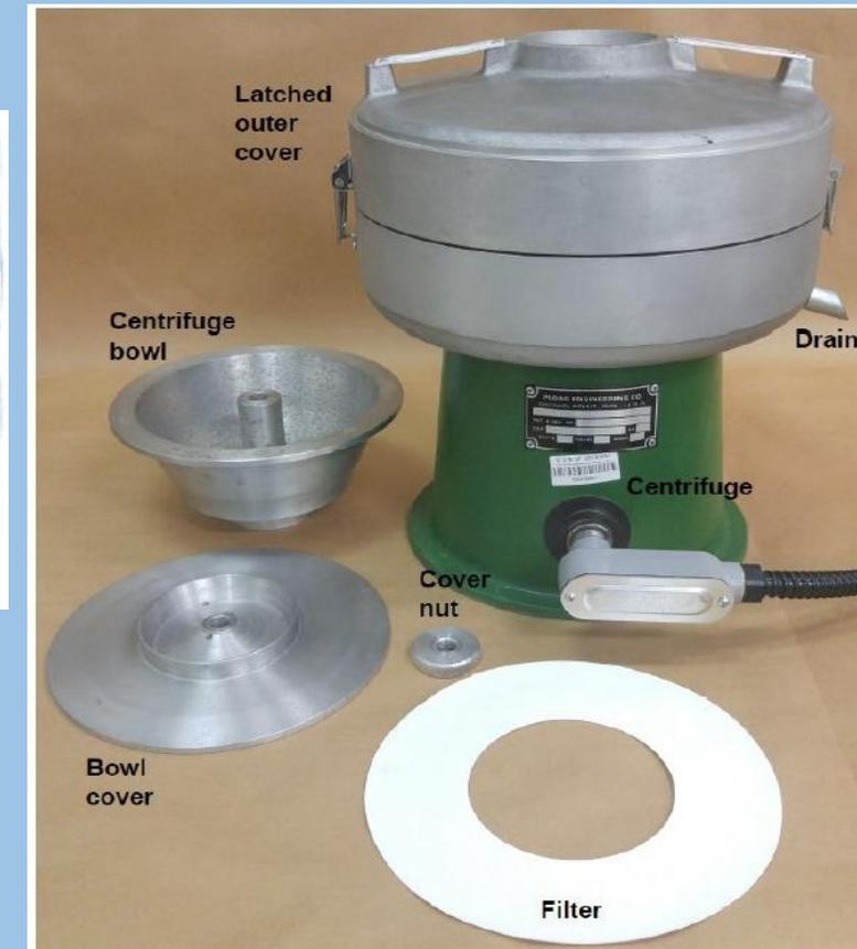
Figure 1—Centrifuge Apparatus (Source: LTRC/DOTD)
