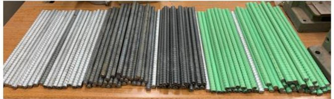
Figure 4. Galvanized, black, ChromX and epoxy-coated bars
