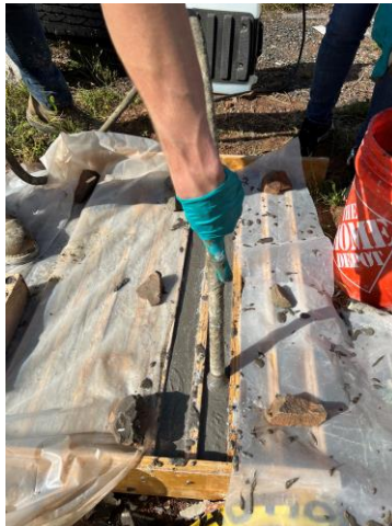
Figure 18. Vibrating the layers of concrete
