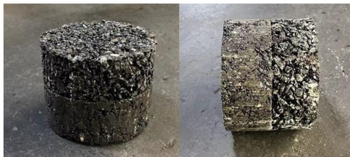
Figure 57. Composite Marshall specimen made with HMA and cold mix
