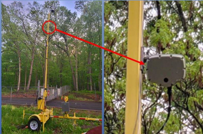
Mobile Trailer with traffic microwave sensor
