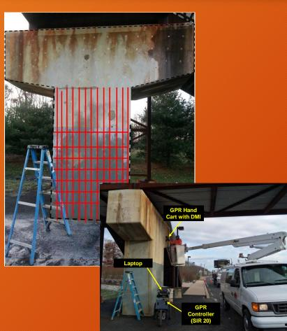
**Rebar Mapping to Complete As-builts**
