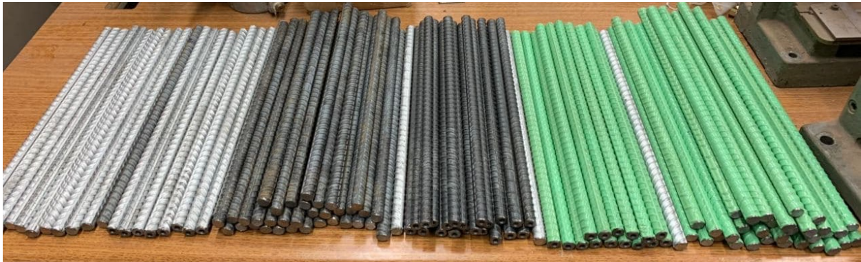
Figure 4. Galvanized, black, ChromX and epoxy-coated bars
