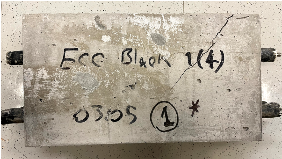
Figure 12. Large shear crack in the failed ECC specimen
