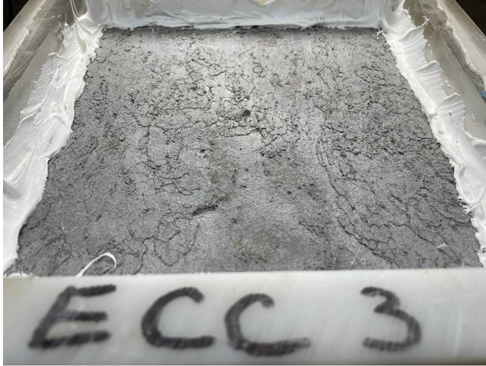
Figure 50. Scaling damage in ECC sample three
