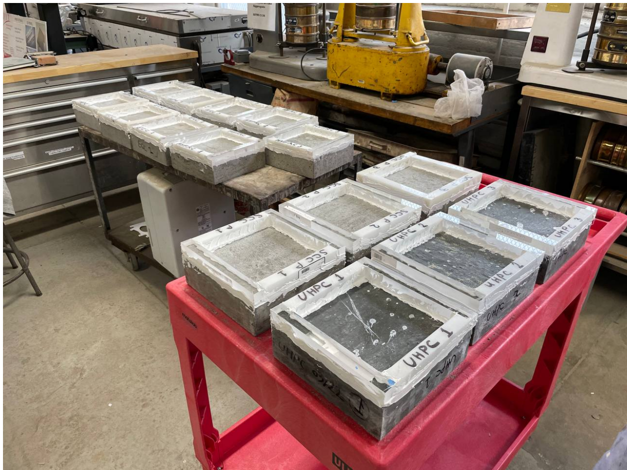
Figure 32. Salt scaling specimens ready to be ponded
