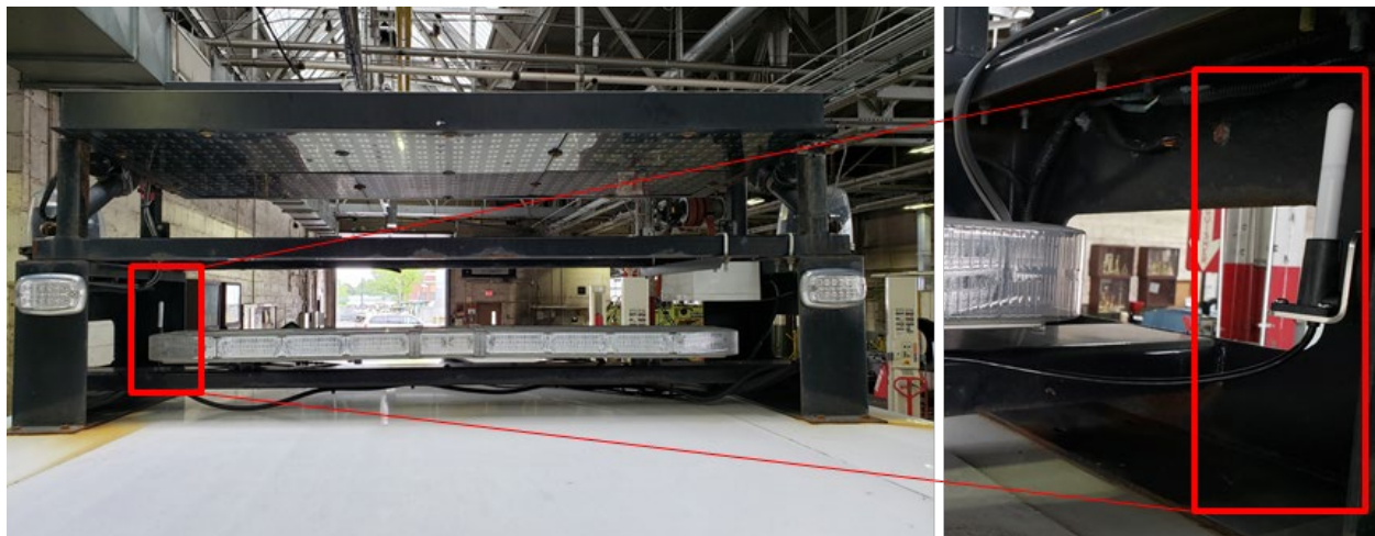
Figure 7. Air temperature and humidity sensor installed on the SSP truck (Source: NJIT)
