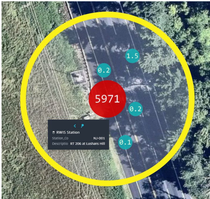
Figure 44. An example of matched MRWIS and RWIS records using a 100 ft buffer and 5-minute data record interval (Source: NJIT)
