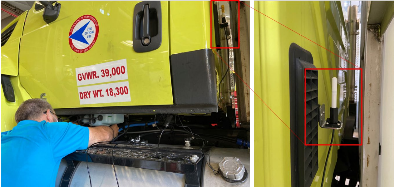
Figure 9. Air temperature and humidity sensor installed on a plow dump truck (Source: NJIT)
