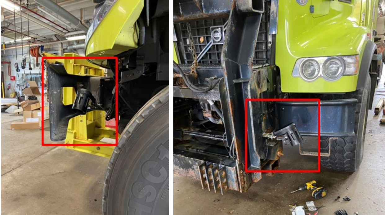
Figure 8. Vaisala MD30 base sensor installed on the plow dump trucks (Source: NJIT)
