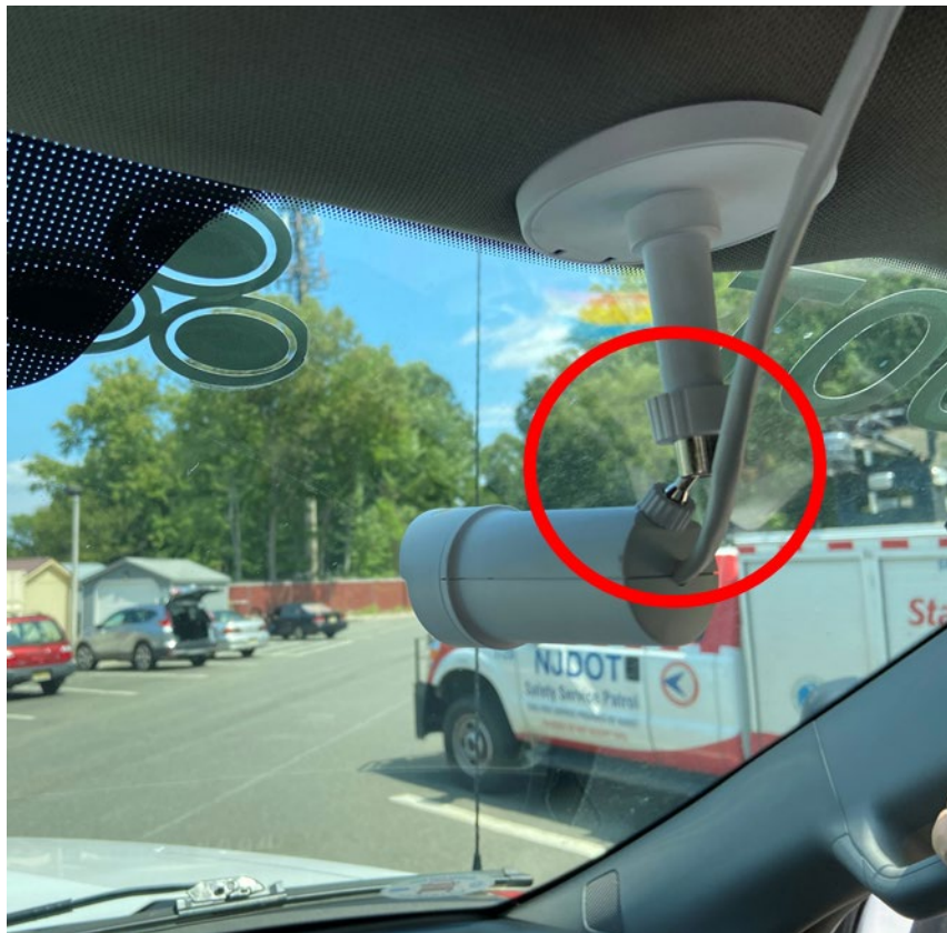
Figure 15. Position of the camera and the camera mount with the tightening bolts circled (Source: NJIT)
