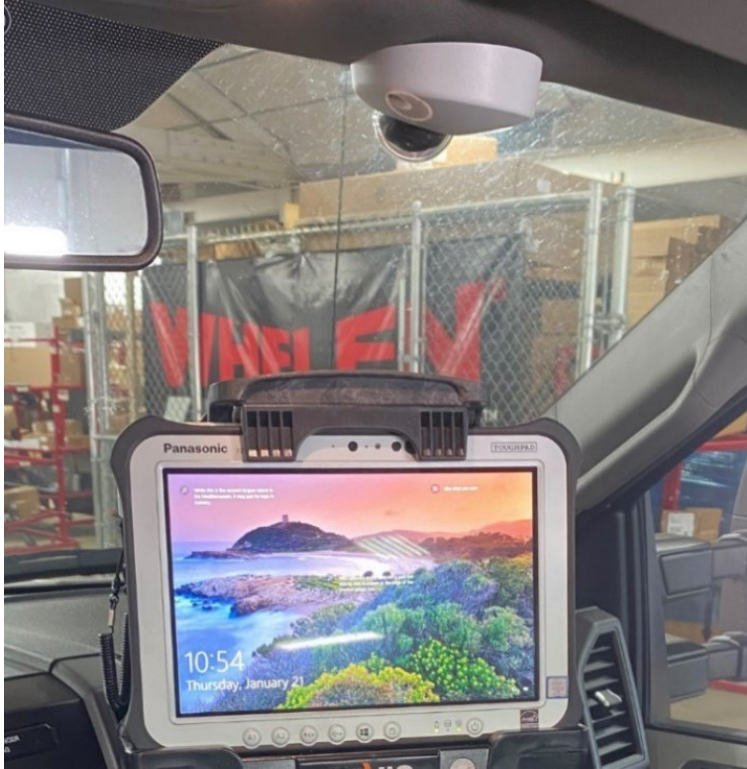
Figure 18. Dome camera (Axis P39 Series) installed in an NJDOT fleet pick-up truck – side view (Source: NJIT)
