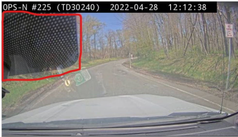
Figure 20. Screenshot of a video stream from windshield camera showing the partial occlusion from the windshield frit (Source: NJIT)
