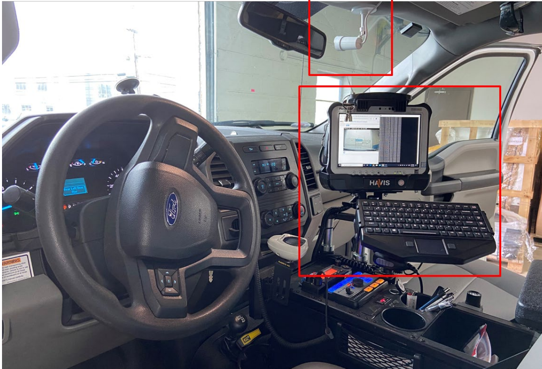
Figure 10. The camera and the computer system installed in an SSP (F-350) truck (Source: NJIT)
