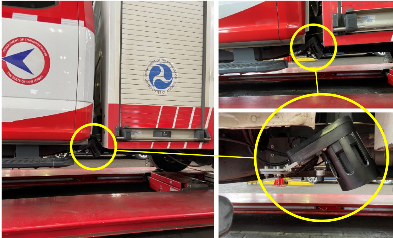
Figure 6. Vaisala MD30 base sensor installed on the SSP truck (Source: NJIT)
