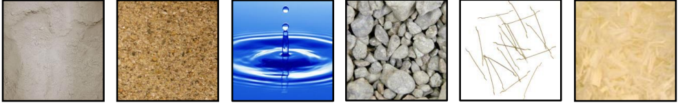
HyFRC - Hybrid fiber-reinforced concrete
