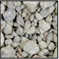
Coarse Aggregate (Crushed Stone)
