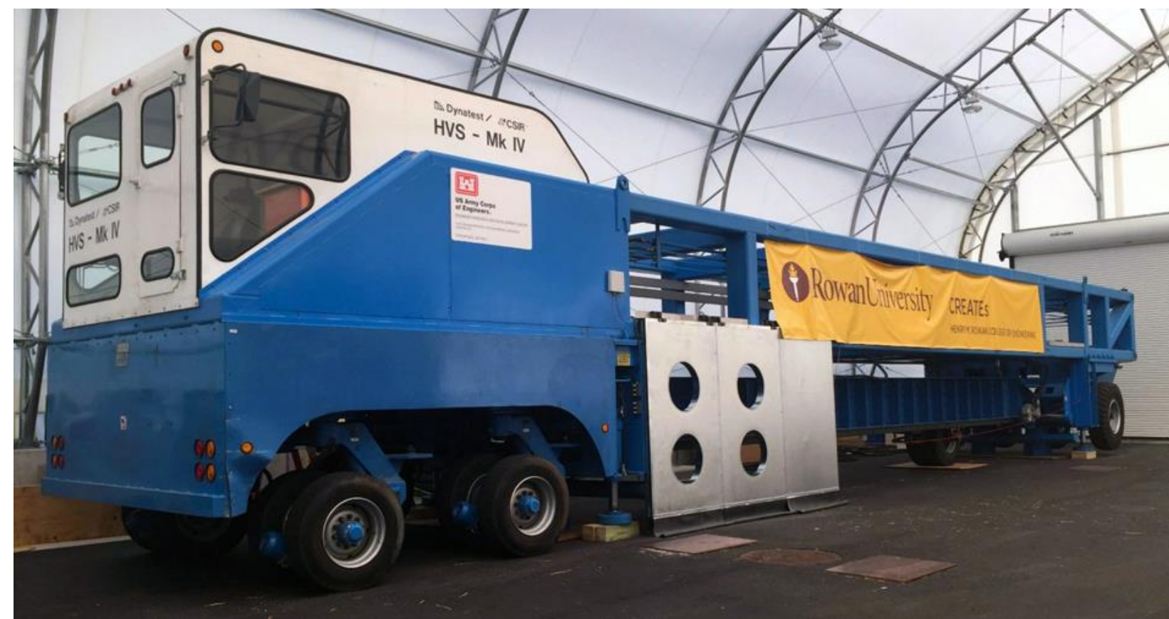
Figure 1 :Rowan University's Heavy Vehicle Simulator (HVS)
