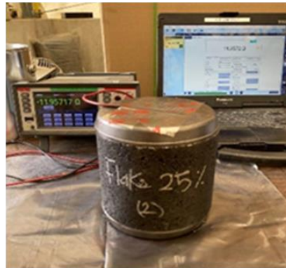
Test resistivity of asphalt sample
