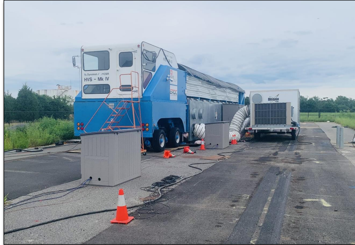
Heavy Vehicle Simulator (HVS) loading in progress
