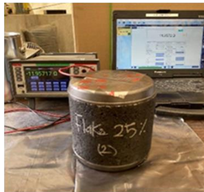
Test resistivity of asphalt sample
