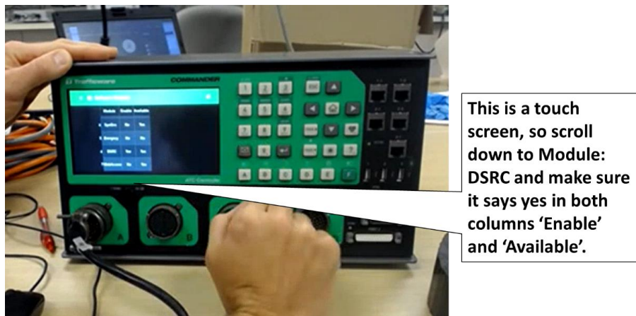
Figure 7. Trafficware Commander Initializing Controller- Scroll to DSRC
