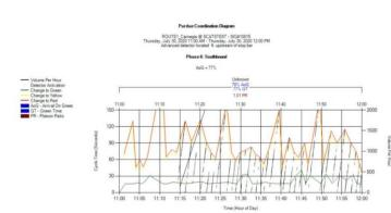
Figure 28. Actual Wavetronix data overlaid on PCD indicating a vector speed (1 hour) for southbound lane 2 at Carnegie and US 1
