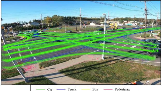
Figure 128. Sample of Road User's Trajectory Results
