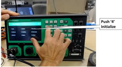
Figure 90. Trafficware Commander Initializing Controller-Initialize
