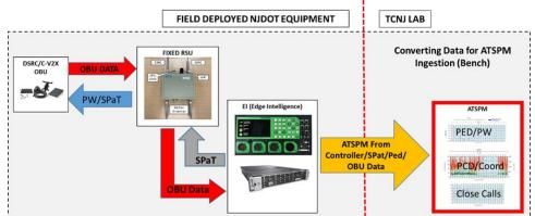
Figure 119. Field Data Collection Setup
