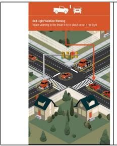
It is a V2I application that the signal phase, timing (SPat), intersection geometry, and position correction information will communicate with the onboard unit, broadcasting warnings for impending red-light violations. RLVW aims to establish a cooperative V2I communication system that prevents drivers from potential crashes at signalized intersections by warning the equipped vehicle if the vehicle is predicted to violate the red light according to current speed and distance.
