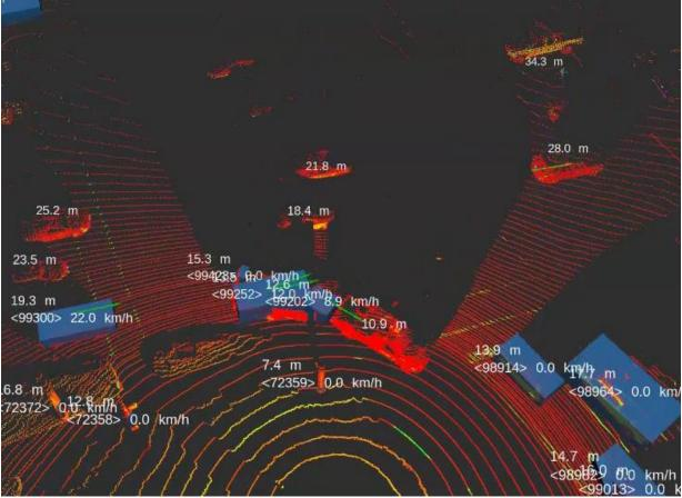
Figure 130. Object Detection Missing Caused by Occlusion
