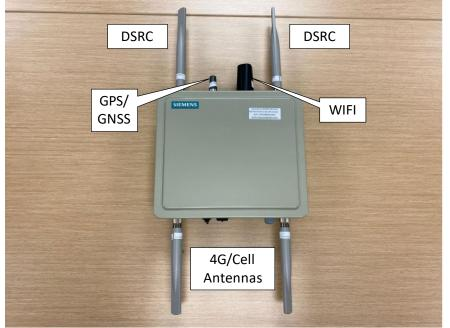
Figure 107. Assembled RSU
