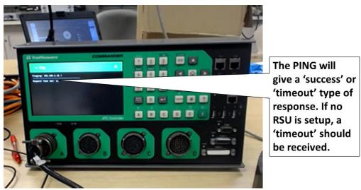
Figure 97. Trafficware Commander Initializing Controller –Ping Test After initialization and all the IP addresses are established, the DSRC needs to be set up. **To set up, up the DSRC, follow this sequence: Home à 6 'Comm' à 9 DSRC Proprietary Setup**
