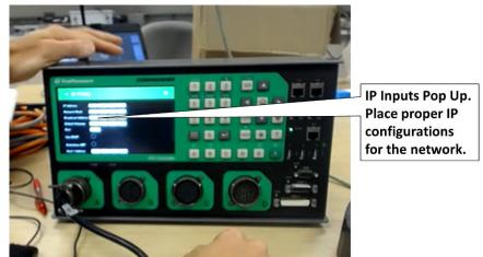
Figure 95. Trafficware Commander Initializing Controller – IPs need to be predetermined
