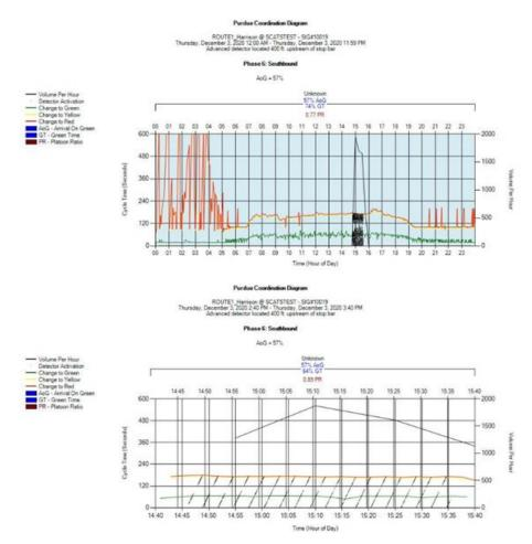
Figure 17. PCDs with Vehicle Arrivals Using Reconstructed Vehicle Trajectories
