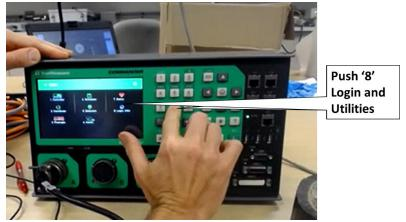
Figure 89. Trafficware Commander Initializing Controller-Utilities
