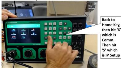
Figure 94. Trafficware Commander Initializing Controller-IP Setup
