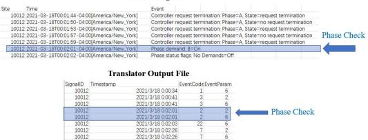
Figure 66. SCATS Log File and Corresponding Event #2 in Translator Output
