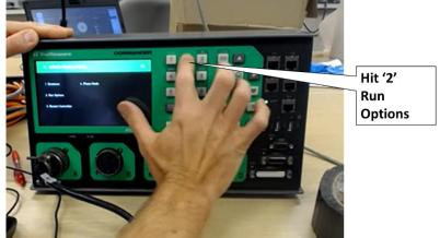
Figure 91. Trafficware Commander Initializing Controller-Run Options
