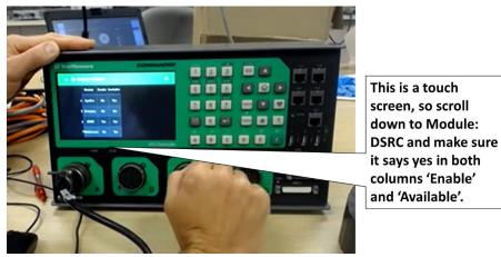
Figure 92. Trafficware Commander Initializing Controller- Scroll to DSRC
