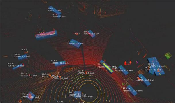
Figure 129. LiDAR Object Detection Results
