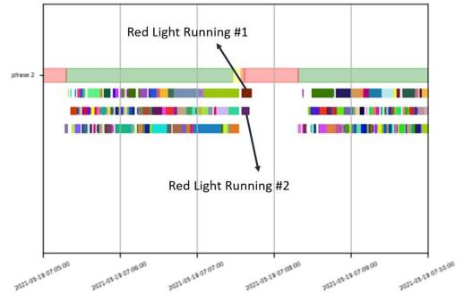
Figure 47. Red Light Running Captured by RCD
