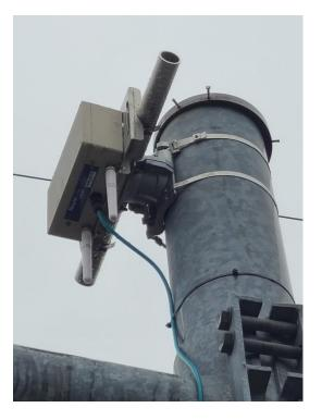
Figure 82. Field Deployed RSU
