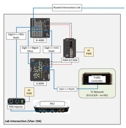
Figure 79. Intersection Level Design
