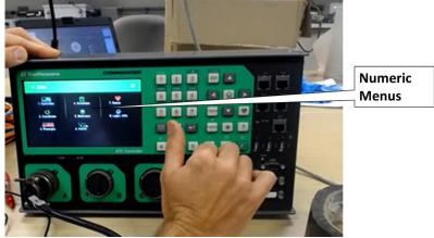
Figure 88. Trafficware Commander Initializing Controller-Numeric Menus
