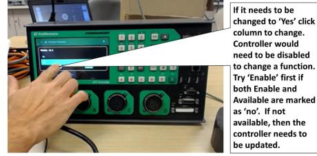
Figure 93. Trafficware Commander Initializing Controller – Assure setup Once the initialization of the DSRC is completed, the controller's IP configuration needs to be set. The Controller will also have the RSU IP address placed in its configuration (Host 2), and the RSU will have the controller IP information. All the IPs must match.: To change the IP follow this sequence. Hit Home à 6 'Comm' à 5 'IP Setup.'
