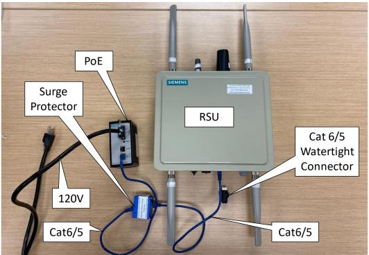
Figure 108. Setup of RSU connections
