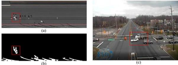
Figure 23. Crossing Vehicle Removal Sample
