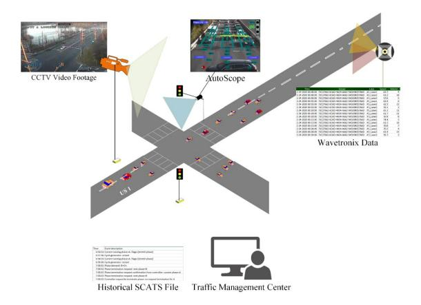
Figure 39. Multi-source Data Collected for Intersection Performance Measurement
