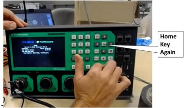
Figure 87. Trafficware Commander Initializing Controller 'Home Key' again if needed.
