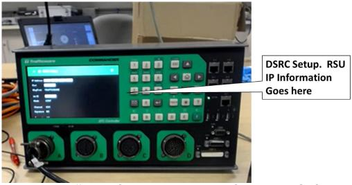
Figure 98. Trafficware Commander Initializing Controller –DSRC setup The following need to be set:
