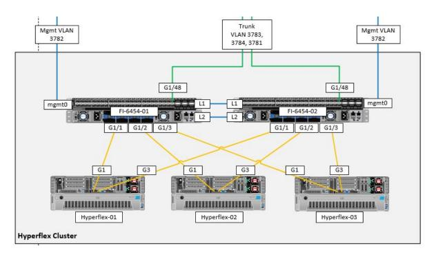
Figure 80. Data Center Level Design
