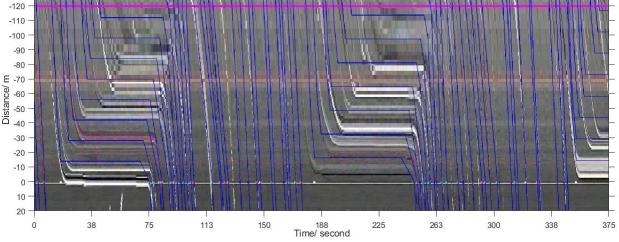
Figure 44. Reconstructed Trajectory and Stop-bar Detector Plotted on STMap
