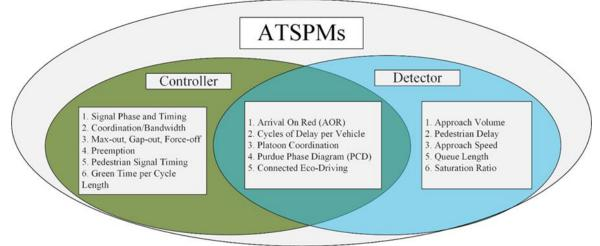
Figure 48. ATSPM Data Source and Performance Measurements
