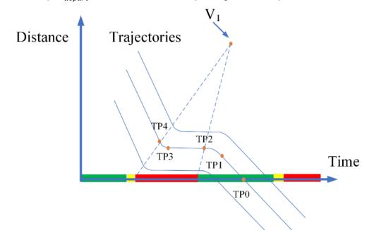
Figure 36. Under-Saturated: Turning Points used for Trajectory Reconstruction
