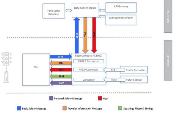
Figure 78. CV Data Flow Architecture
