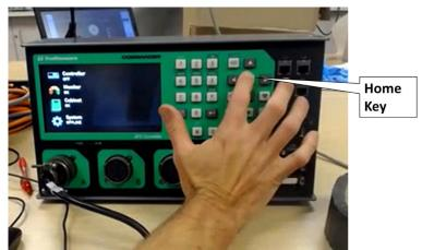
Figure 86. Trafficware Commander Initializing Controller 'Home Key'
