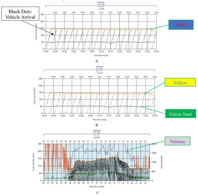
Figure 45. Purdue Coordination Diagram Using Reconstructed Trajectory. A. PCD with Ground Truth Advanced Detection. B. PCD with Algorithm Advanced Detection. C. 24hour PCD with Algorithm Reconstructed Trajectory.
