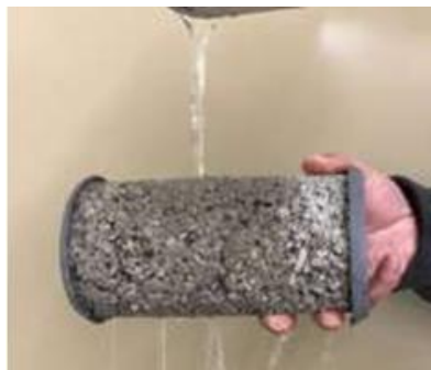
Water draining through porous concrete
