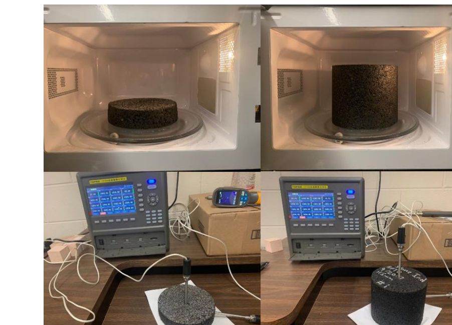
Fig. 5. Microwave heating test
