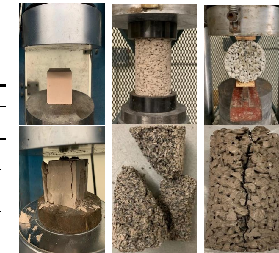
Fig. 3. Mechanical test setup and failure specimens
