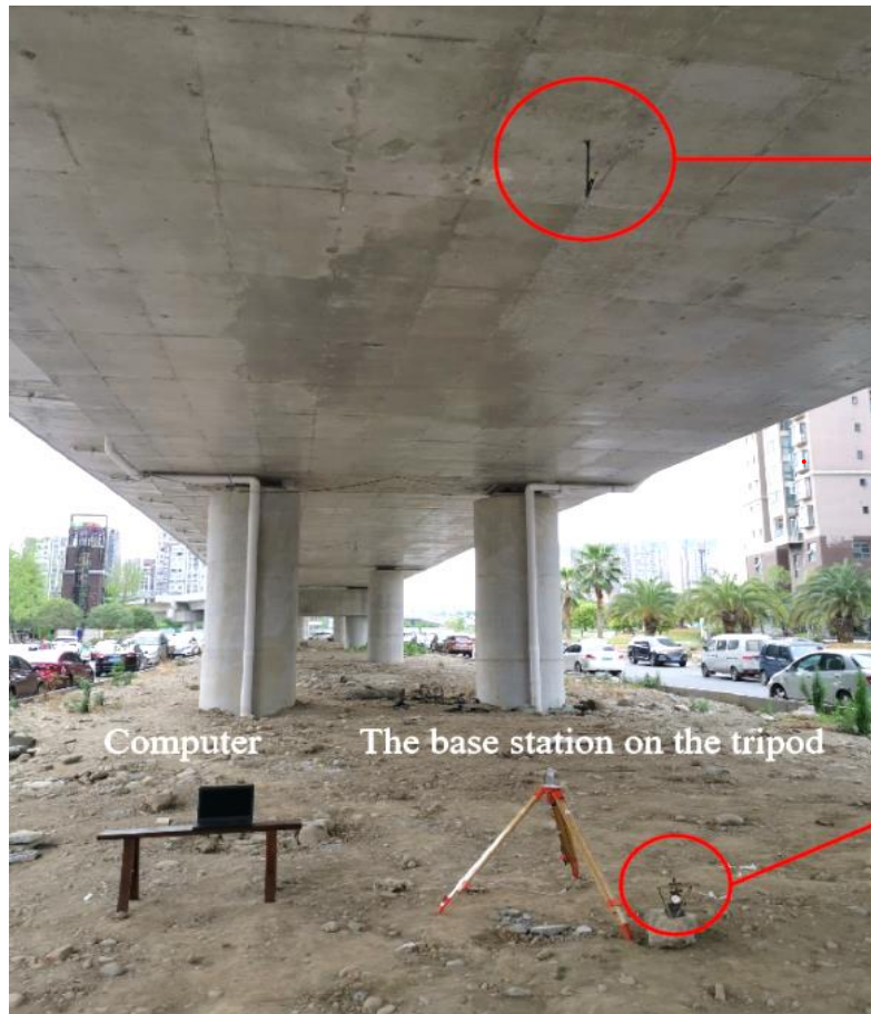
The target node fixed on the bottom of the bridge
