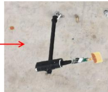
The target node fixed on the bottom of the bridge
