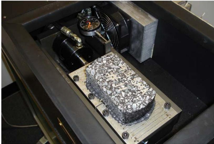
**Figure 15 – Picture of the Overlay Tester (Chamber Door Open)**
