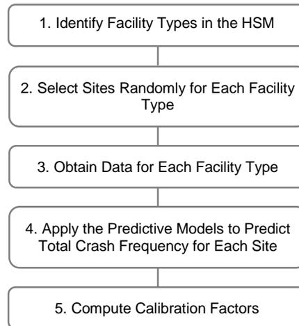
**Figure 1.** Calibration process recommended by the HSM <sup>(2)</sup>
