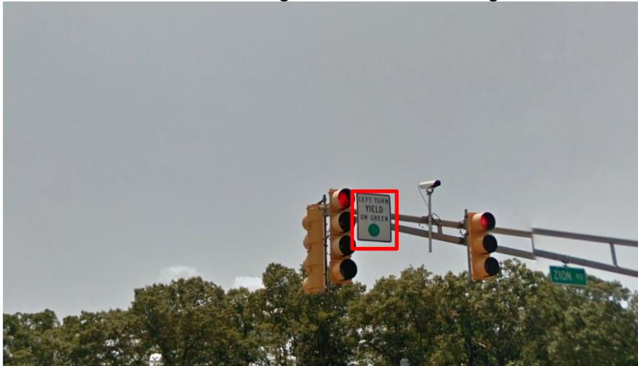
**Figure 47:** A sign indicating that left-turns are allowed on green
