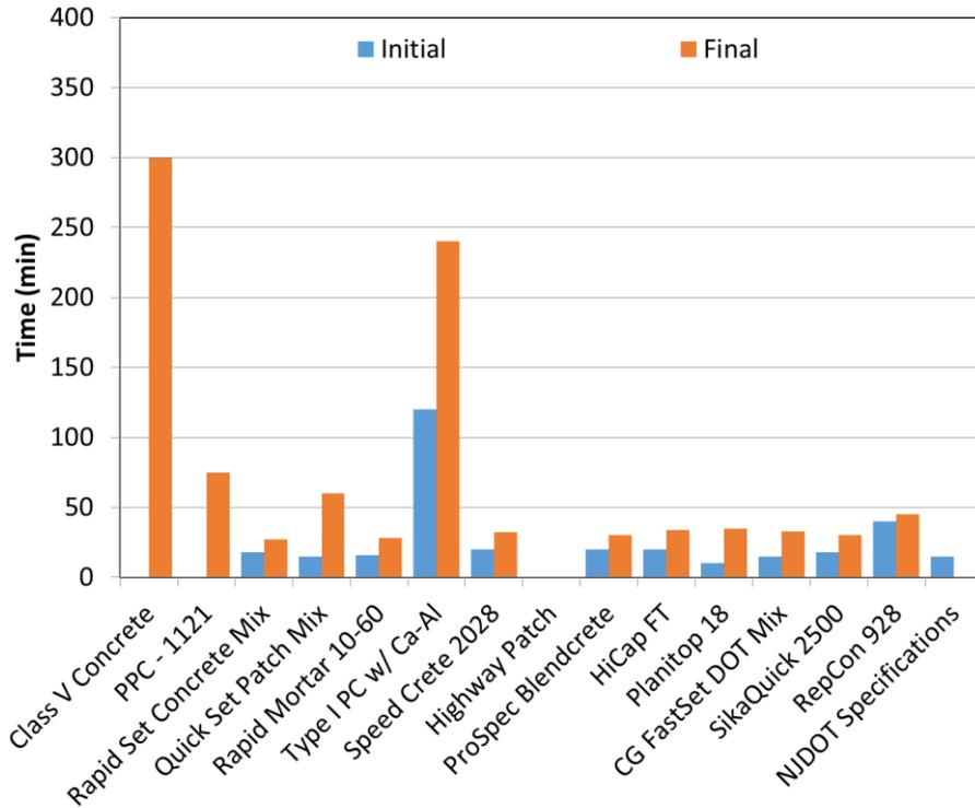
**Figure 22: Setting Time of CIP Rapid Repair Mixtures**
