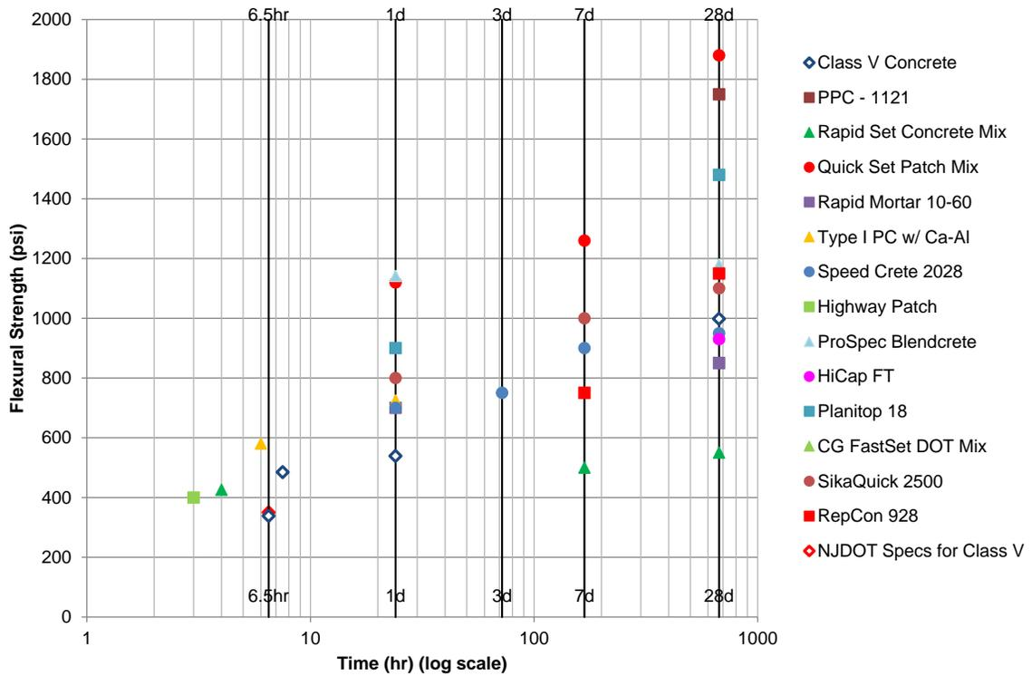
**Figure 21: Flexural Strength of CIP Rapid Repair Mixtures**
