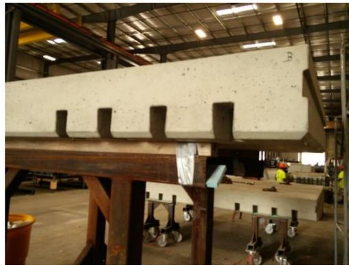
**Figure 10: Fort Miller bottom-slot dowel system.**
