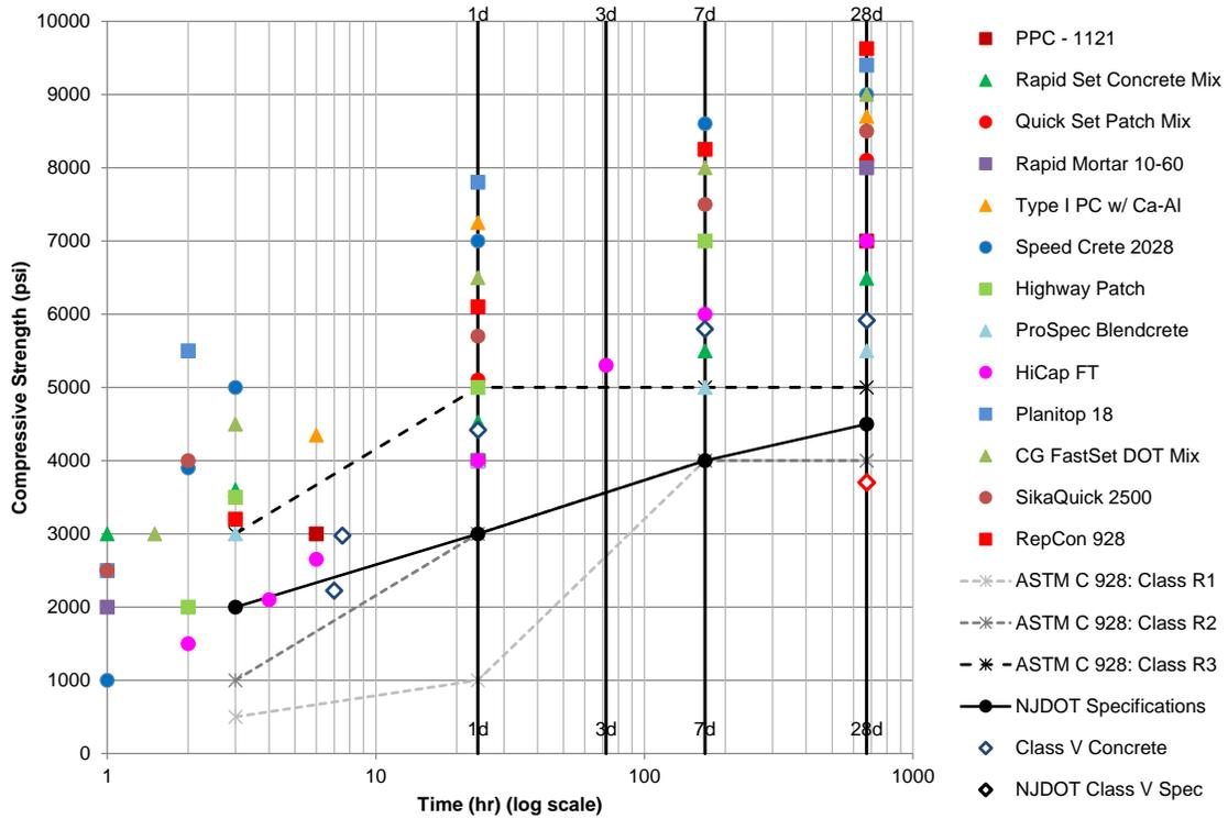
**Figure 20: Compressive Strength of CIP Rapid Repair Mixtures**
