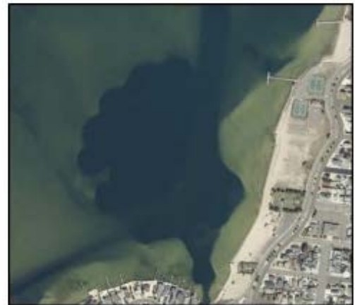
A cusped boundary created by a dredge can be seen on the northern and eastern limits of Dredged Hole 25 in 2012 aerial photograph.
