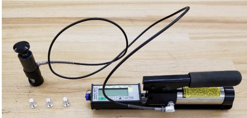
Figure 7. Pull Off Tester and 20 millimeter Pull Off Dollies
