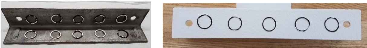
Figure 3. Specimen preparation: Attachment of O-rings using water soluble glue and their removal after the curing of the coating.
