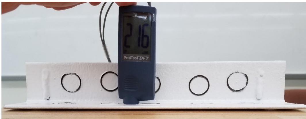
Figure 13. Thickness gage used for measuring the thickness of paint layers
