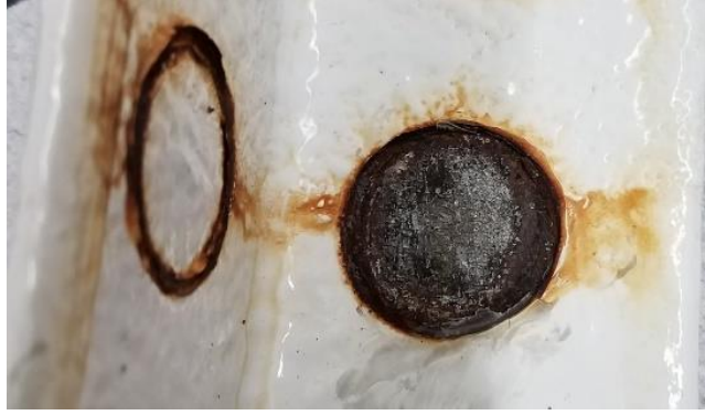
Figure 9. Images of circular coating: Before and after pull off test
