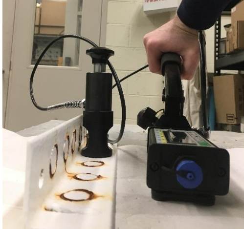
Figure 14. Typical Pull Test
