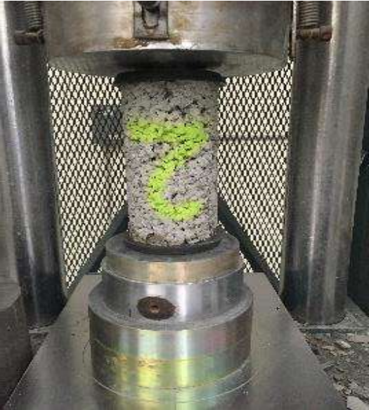
Figure 6. Compressive strength test on 4"x8" sulfur capped cylinder
