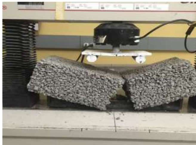
Figure 9. Flexural failure of porous concrete beam
