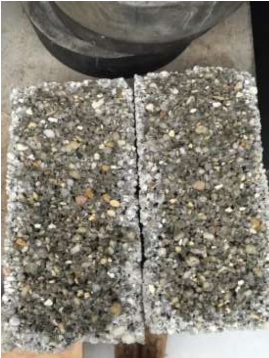
Figure 12. Splitting tensile test failure of porous cylinder
