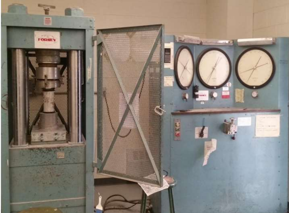
Figure 11. Testing machine used for the splitting tensile strength tests
