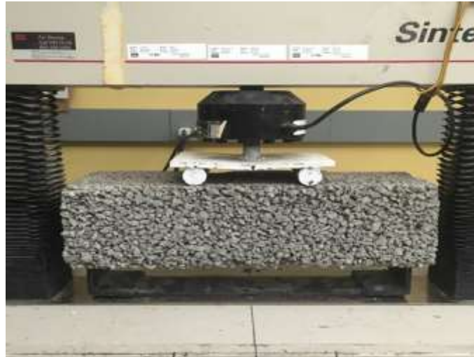
Figure 8. Porous concrete beam during flexural test (6"x6"x18" beam)
