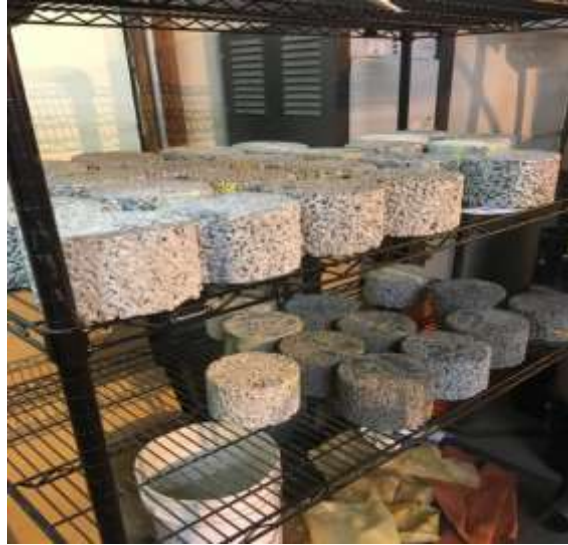
Figure 22. Sample cuts from 6 in x 12 in pervious concrete cylinders used for air void and permeability measurements
