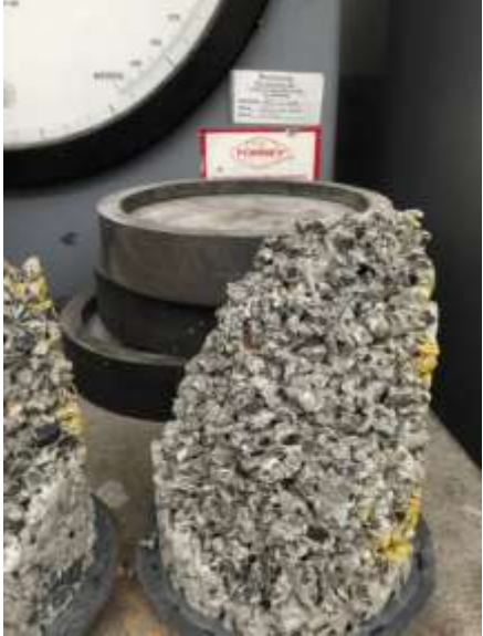
Figure 7. Failure of 4 in x 8 in pervious concrete cylinder in compression
