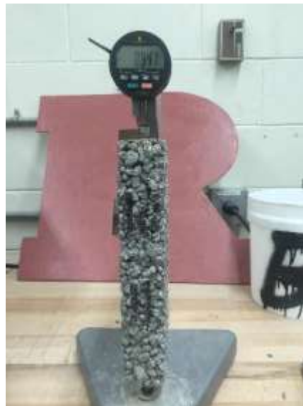
Figure 14. Porous concrete prism placed in comparator for free shrinkage test
