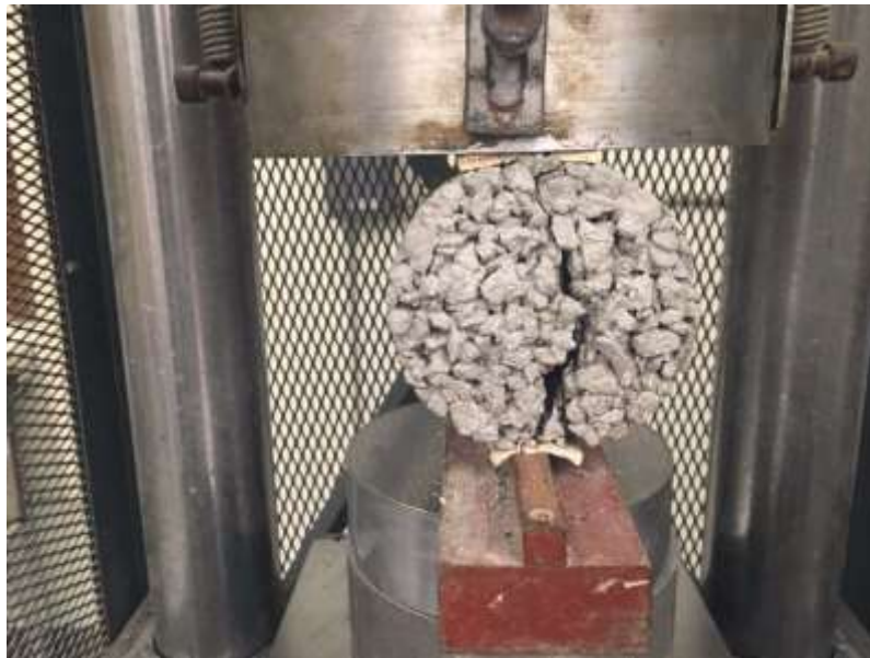
Figure 10. Splitting tensile strength test of 4"x8" porous concrete cylinder
