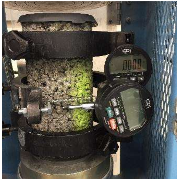
Figure 13. Elastic modulus test of 4"x8" sulfur capped porous cylinder
