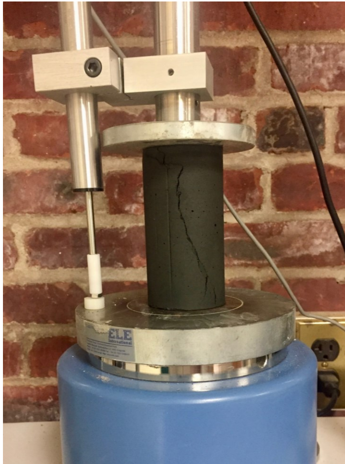
Sample undergoing UC testing on ELE device
