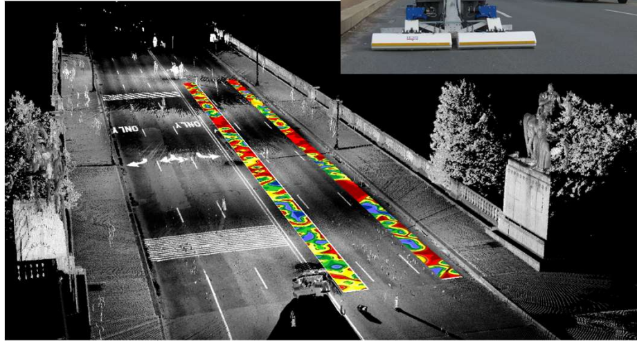
Superimposed RABIT's Impact Echo Data on LiDAR Image of Arlington Memorial Bridge
