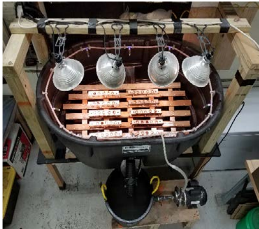
Cyclic Weathering Test-Chamber used for Accelerated Testing
