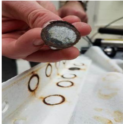
20 Millimeter Pull Off Dolly: After Pull Off Test
