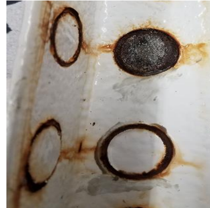
20 Millimeter Pull Off Dolly: Over Coat Paint Removed After Pull Test
