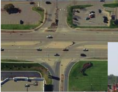
This intersection design restricts left-turn movements to improve safety.
